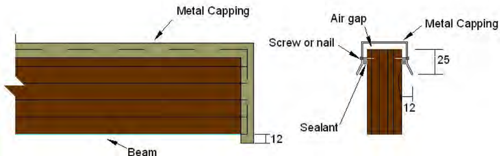
Figure 12: Beam capping / end flashing
