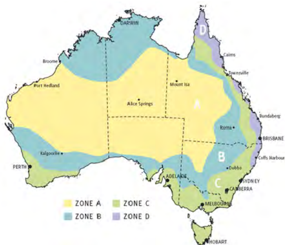
Figure 3: Above-ground decay hazard zones for Australia (Zone A has least and Zone D greatest potential for above-ground decay) Ref: Timber Service Life Design Guide, FWPA 2007
